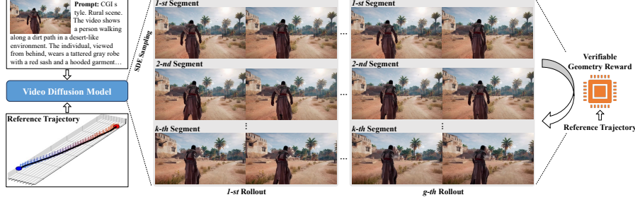
Fig. 3: Framework of CAMVERSE. Given the input first frame, a text prompt, and a reference camera trajectory, the video diffusion model \pi_\theta samples G rollouts by a stochastic reverse process (SDE sampling). Each rollout is partitioned into non-overlapping segments. For each rollout, a large 3D model is used to estimate the camera trajectory. After aligning the generated trajectory to the reference one, the verifiable geometry reward compares each pair of generated-reference segments in a relative manner and assigns a dense alignment score. With this type of reward signal, we conduct GRPO fine-tuning, improving camera-control accuracy and geometric consistency.
