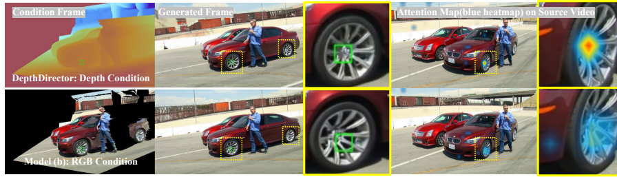
Fig. 11: Attention visualization. Green box marks the query noise patch; the heatmap shows how source video patches attended by it. We normalize weight by a factor(0.04), red means higher. DepthDirector maintains strong and precise attentions to corresponding patch from source video, producing consistent outputs, while the RGB variant produces weak and rough attentions, leading to distorted structures.
