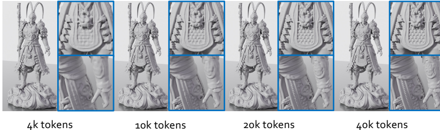
Fig. 6: Qualitative test-time scaling with respect to token budget. Increasing the number of tokens at inference time progressively improves reconstruction quality, enabling more faithful recovery of fine-grained geometric details.
