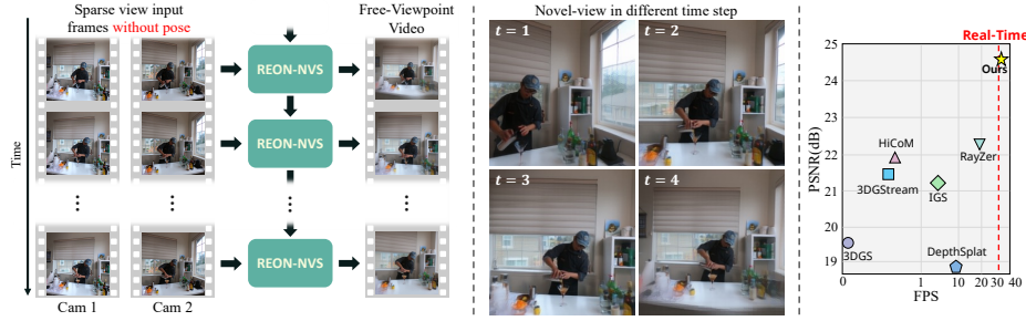
Fig. 1: We present REON-NVS, a feedforward online NVS framework that performs pose estimation and novel-view reconstruction from sparse-view video streams in real-time. The right figure is evaluated on the Neural 3D Video [20] dataset.
