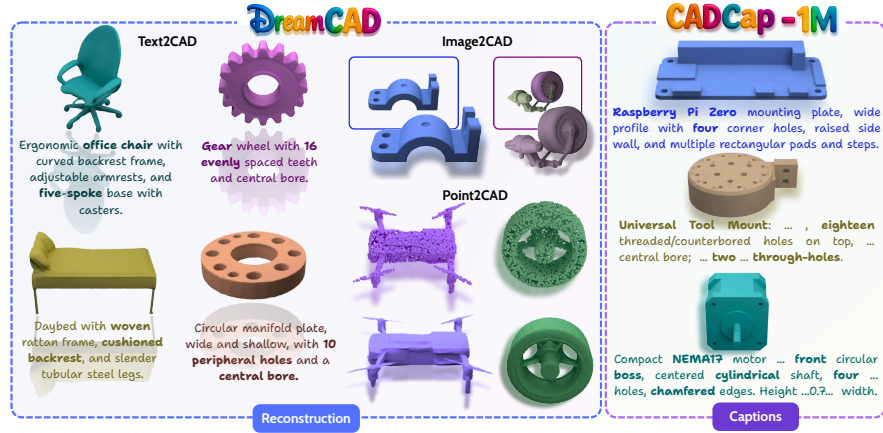
Fig. 1: Our proposed DreamCAD (left) is a multimodal generative framework that can reconstruct CAD models from text, images, and point clouds using parametric patches. CADCap-1M (right) provides 1M+ GPT-5-generated captions.
