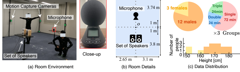
Fig. 6: Experimental setup. (a,b) Our measurement environment consists of a set of speakers and a microphone for active acoustic sensing, along with motion capture cameras to obtain ground-truth poses. (c) Our AMP dataset consists of 12 male and 3 female participants, with heights ranging from 150 cm to 181 cm. The participants were divided into three groups. For each group, we collected 72 minutes of single-person data, 24 minutes of double-person data, and 24 minutes of triple-person data.
