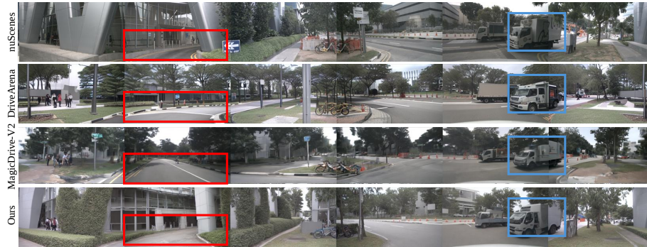
Fig. 4: Qualitative comparison of generated samples under nuScenes [6] validation conditions. Using the same nuScenes conditions, we generate multi-view images with each method to evaluate visual quality. Compared to the ground truth (top row), MagicDrive-V2 [15] produces structural artifacts in road conditions (red boxes), and DriveArena [93] exhibits view-inconsistent object shapes (blue boxes). Our method better preserves scene layout while maintaining superior multi-view consistency.
