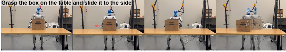
Fig. 7: Humanoid Policy Rollout. The robot grasps a box on the table with both hands, squats down, and steps to the right.
