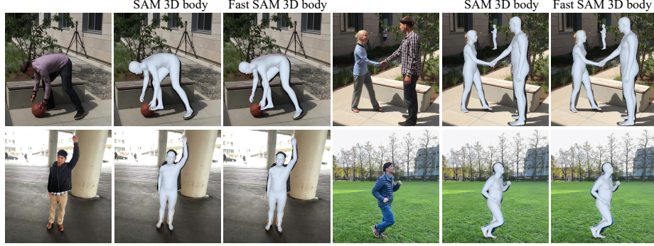
Fig. 4: Qualitative comparison. The original SAM 3D Body (left) and our Fast variant (right) yield visually comparable mesh reconstructions across diverse poses and multi-person scenes on 3DPW [38] and EMDB [19].
