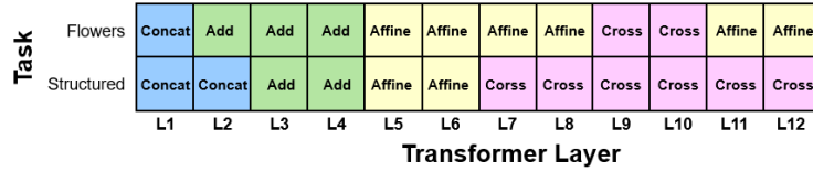
Fig. 4: Task-specific fusion preferences. The discovered operator distributions differ between Flowers and Structured tasks: early layers consistently favor lightweight fusion ( Concat/Add ), while deeper layers shift toward semantic operators ( Affine/Cross ), revealing task-specific adaptation patterns.
