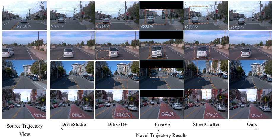
Fig. 4: Qualitative comparisons on WOD [40]. Our method and Difix3D+ [54] use renderings of DriveStudio [10] for camera control and restoration, respectively. Note that the officially released FreeVS [47] model is trained and tested on a cropped resolution that excludes sky regions to reduce computation and avoid LiDAR-sparse areas.
