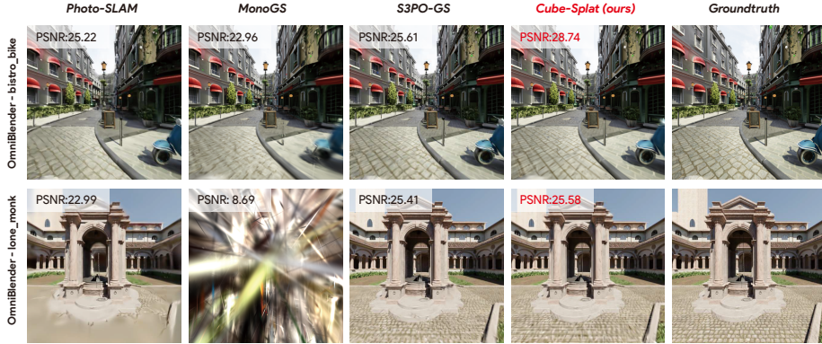
Fig. 5: Qualitative comparison of outdoor rendering results. Novel view synthesis on OmniBlender outdoor scenes. Compared to baselines that suffer from blurring or catastrophic map failure (e.g., MonoGS [26] in the bottom row) in unbounded environments, Cube-Splat generates cleaner reconstructions with sharper structural details.
