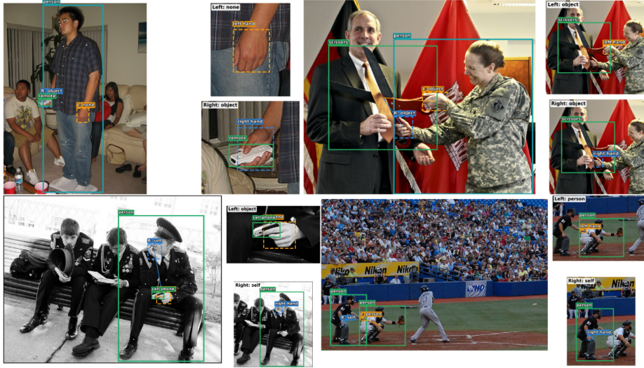
Fig. 1: Visualization examples from our person-centric bi-manual interaction dataset. For each person instance, we annotate a human bounding box, body keypoints, left/right hand regions, hand contact states, and the corresponding interaction targets. In each example, the full image is shown together with zoomed-in views of the left and right hands to highlight fine-grained hand-object interactions. Dashed boxes indicate hand regions, solid boxes indicate interaction targets, and the annotations explicitly preserve left/right hand ownership under a shared human instance.
