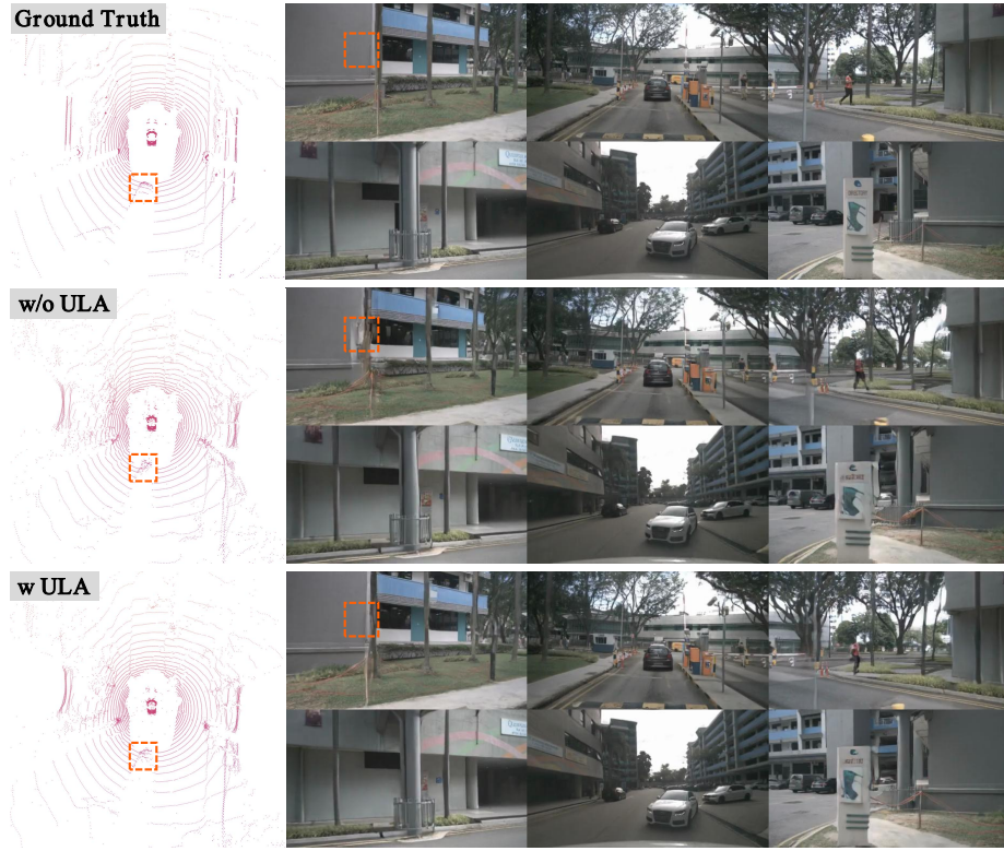
Fig. 8: Qualitative comparison of generated outputs with and without the Unified Latent Anchoring (ULA) module. The top row displays the ground truth. The middle row illustrates results without ULA, highlighting geometric inconsistencies and cross-modal misalignment between LiDAR points and RGB content. The bottom row presents results with ULA, showing enhanced cross-modal geometric coherence and improved visual quality.
