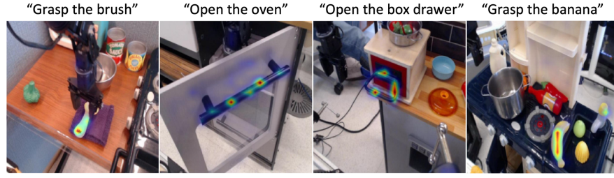
Fig. 7: Zero-shot Espresso-2D on real-world robot scenes. Despite the visual domain gap from Objaverse renderings, Espresso-2D pretrained on Affogato-750K localizes open-vocabulary affordances correctly across diverse, cluttered Open X-Embodiment [53] robot workspace images.
