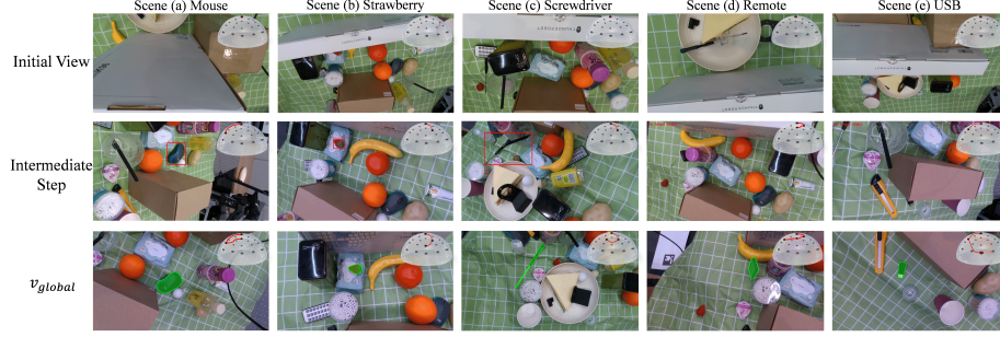
Fig. 3: Stage I: Global View Exploration. Columns correspond to five cluttered real-world scenes (a–e) in Table 2. Rows show the progression from the initial arbitrary view (top), to intermediate exploration (middle), and the final selected Next-Best-View v_{\text{global}} (bottom), which exposes the target for initial grasp hypothesis.
