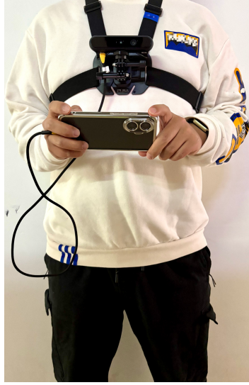
Fig. 2: Illustration of the data collection equipment. We fix the RGB-D sensor to the chest with a shoulder strap and attach it to an Android smartphone.
