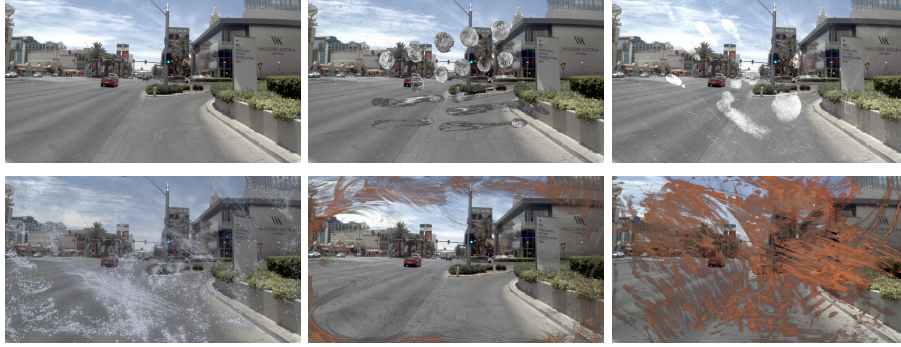
Fig. 4: Example of synthetic sensor corruptions applied to the front-center camera. From left to right, top to bottom: Nominal, Fingerprints, Handprints, Frost, Mud (Mild), Mud (Heavy).
