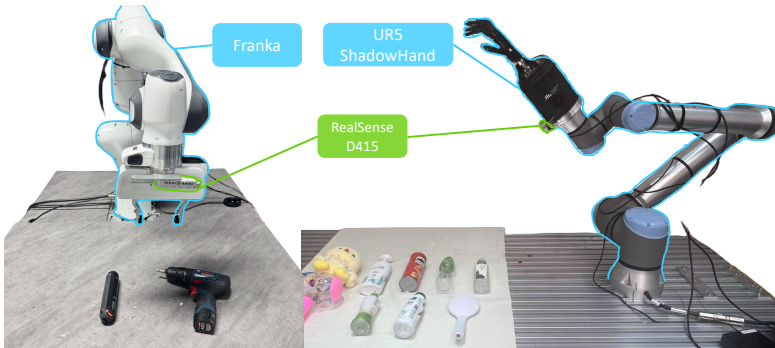
Fig. 5: Object Manipulation robot setup.
