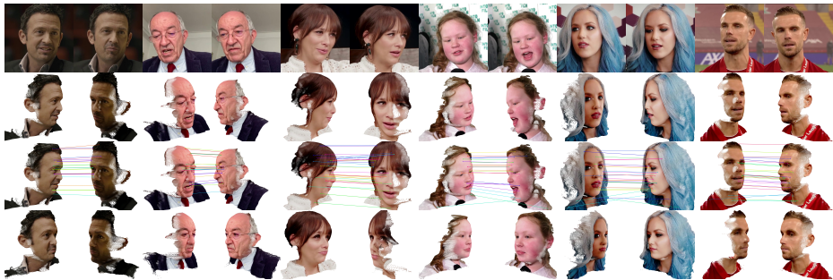
Fig. 1: Face Anything. Unified 4D facial reconstruction and dense tracking from image sequences via joint prediction of depth and canonical facial coordinates. Top to bottom: RGB input, reconstructed geometry, correspondences, and canonical points.
