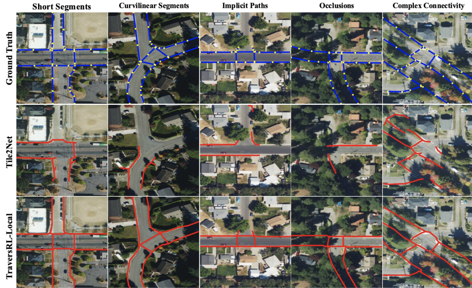
Fig. 1: Qualitative examples of pedestrian pathway generation. Representative aerial intersection scenes illustrating common challenges for pedestrian mapping: {short segments, curvilinear segments, implicit paths (no crossing marks), occlusions from trees, and complex connectivity}. Top: ground-truth graph (blue; yellow dots mark vertices). Middle: predictions from the state-of-the-art segmentation-based method, Tile2Net (red). Bottom: predictions from our TraversRL-Local model (red). These examples highlight the topology-sensitive nature of pedestrian networks, and demonstrate TraversRL’s robust generation across diverse real-world challenges.
