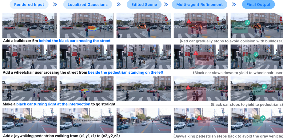
Fig. 1: Overview of SIMSplat. Our framework enables language-guided, fine-grained editing in driving scenarios. Based on human/VLM-generated prompts, it first queries related objects from the Gaussian scene, then performs editing followed by multi-agent path refinement, ensuring the final scene remains realistic and consistent across all agents. SIMSplat supports a wide range of editing operations covering both vehicles and pedestrians. The red/green areas indicate potential collision and refined regions.
