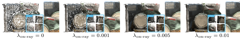
Fig. 6: Ablation of the on-ray regularizer with different weights. For each weight, we show the predicted surface points in 3D (left), the corresponding UV coordinates in the 2D atlas (middle), and the final rendered texture from texture maps (right). As shown, the on-ray loss ensures a better coverage of the surface, which leads to more uniform UV coordinates and gives a sharper texture in the renderings.
