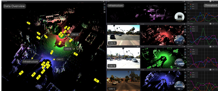
Fig. 1: COOPERSCENE sample data visualization. Left: Overlay of point clouds from all agents (three connected autonomous vehicles (CAVs) in red, green, blue, and infrastructure in purple) with global 3D object labels (yellow). Middle: Individual agent sensor views in local frames. Right: Real time C-V2X throughput measured between all agent pairs.
