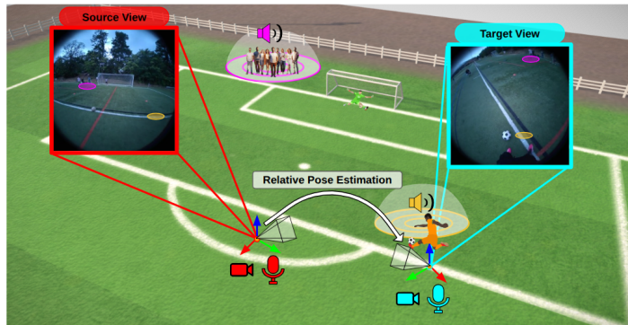
Fig. 1: Main idea: we propose to estimate relative camera pose from in-the-wild videos using both vision and multichannel audio. Unlike traditional active echolocation sensing, our model relies only on passive scene audio—gaining spatial cues opportunistically from naturally occurring ambient and foreground sound sources.
