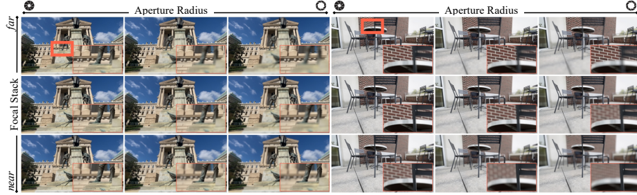
(b) Example data rendered from reconstructed light fields. Rows vary the focal plane to bring different scene depths into focus. Columns vary the aperture radius to control defocus strength.
