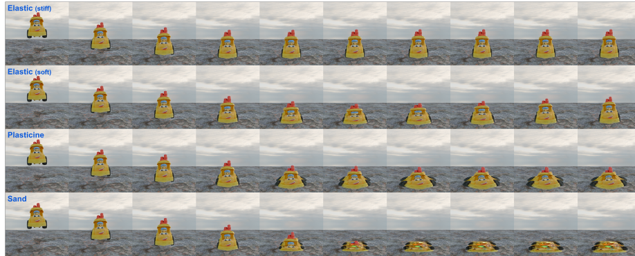
Fig. 5: Generalization to novel materials. Elastic (stiff): E=10^7 , \nu=0.49 . Elastic (soft): E = 8000 , \nu = 0.4 . Plasticine: \tau_Y=500 . Sand: \theta_f=10^\circ .
