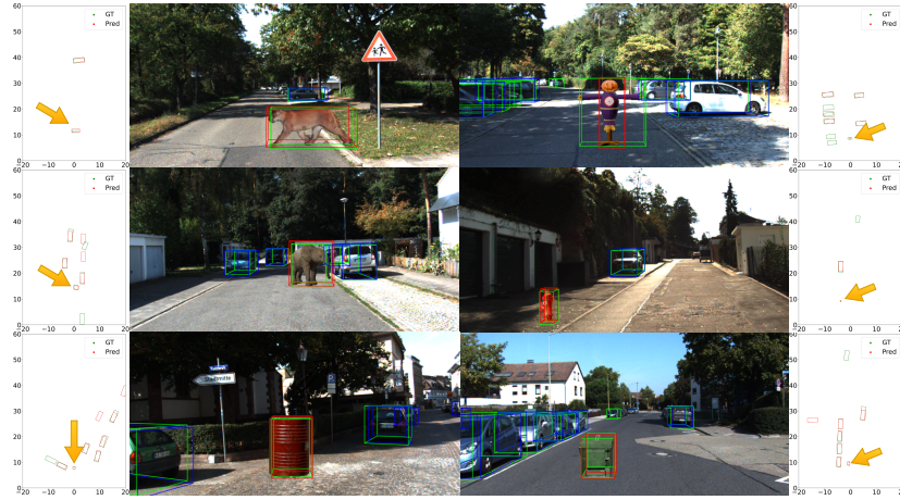
Fig. 5: Visualization results with 3D boxes and BEV map. In the RGB images, red 3D boxes represent predicted anomaly categories, blue 3D boxes represent predicted known categories, and green boxes indicate the ground truth.
