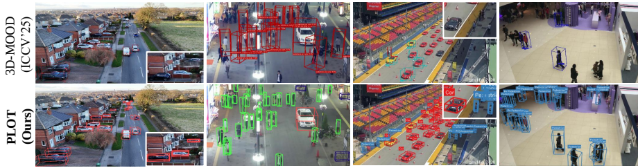
Fig. 1: Zero-shot estimation on MOT17 [34] and Pexels [8]: Predictions from (top) an open-set M3OD model [55] and (bottom) our pseudo-labeling method. Our method performs well on out-of-domain camera views (zoom in for a better view).
