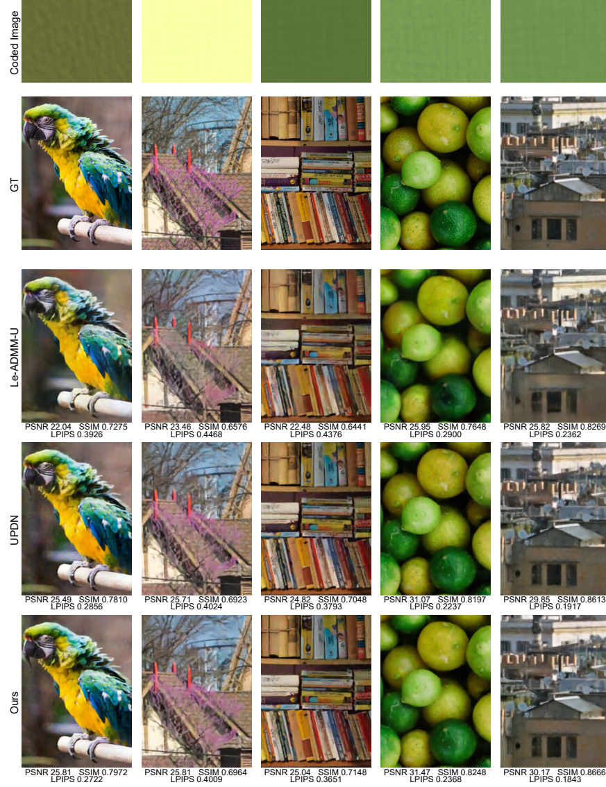
Fig. 6: Qualitative comparison of reconstruction results on real-world data. We compare EK-DUN with Le-ADMM-U, a baseline unrolled network with a shift-invariant PSF, and UPDN, a state-of-the-art unrolled network with multiple learned PSFs. EK-DUN achieves high-fidelity reconstruction comparable to UPDN, preserving fine details and reducing artifacts in challenging regions.
