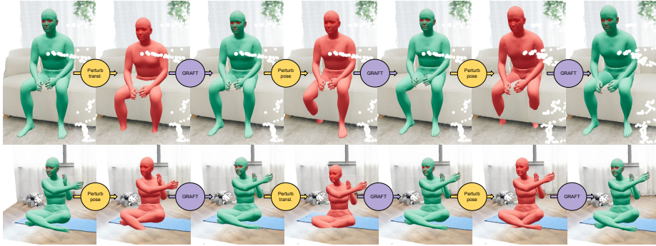
Fig. 3: GRAFT as a learned HSI prior. Starting from an initial state (green mesh), we apply translation and pose perturbations (red); after each perturbation, GRAFT—operating with no visual features —projects the state back to a geometrically valid human–scene interaction (green). Our geometric probes encode contact and penetration cues that drive each correction step. We refer readers to the supplementary video for a comprehensive visualization.
