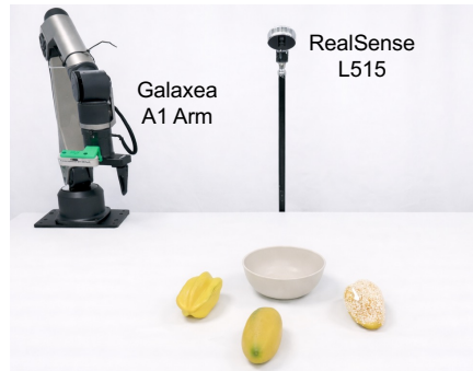
Fig. 7: Real-world setup for Galaxea A1 Arm Platform.
