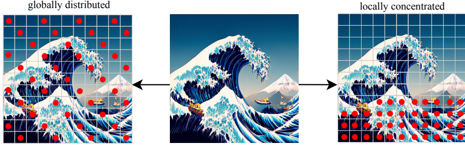
Fig. 3: Comparison between periodic gradient sampling in GSGR and conventional end-segment gradient recording. Traditional practices collect gradients only from the final portion of the sequence, leading to redundant adjacent signals. GSGR instead samples gradients at regular intervals across the trajectory, capturing broader context with reduced redundancy.
