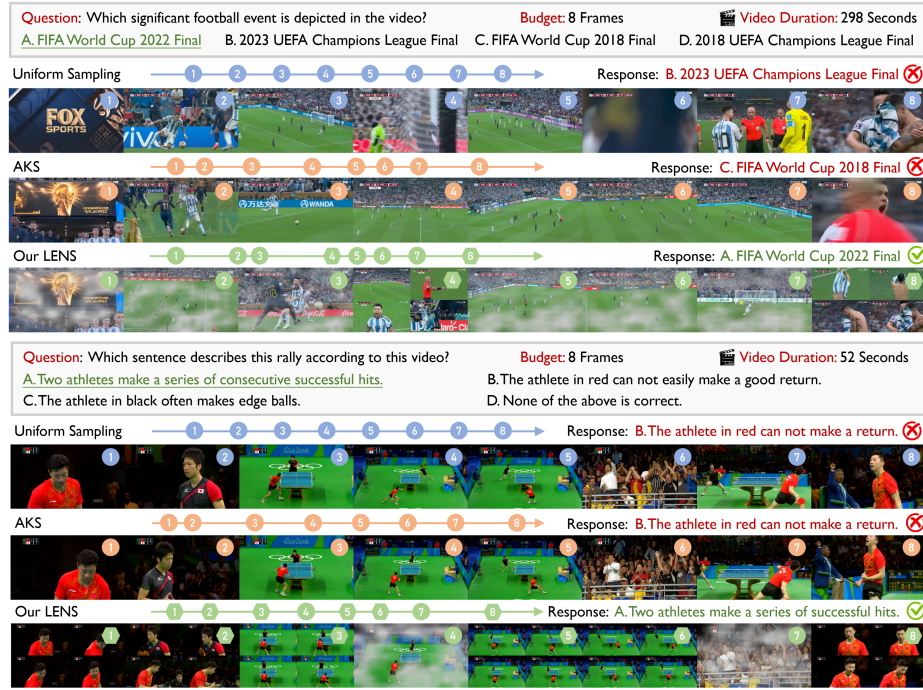
Fig. 3: Qualitative comparison on two representative samples from the Video-MME benchmark [10]. The selected frames from LENS are compared against those obtained via uniform sampling and AKS [31]. Note that frames obtained via spatial zoom-in are denoted by green circles, while those from temporal zoom-out are represented by green hexagons.
