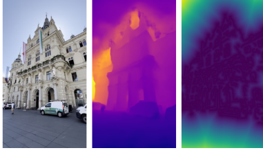
Fig. 2: Example of input RGB image, VGTT raw depth, and the corresponding DTF.
