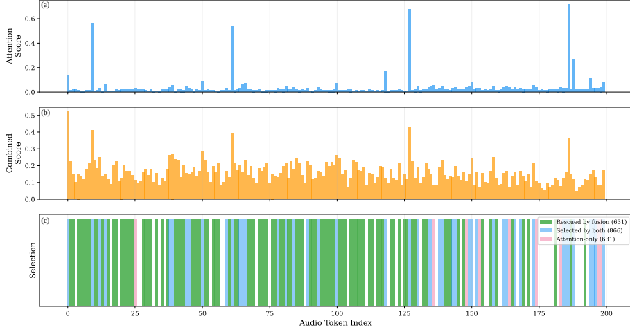
Fig. 2: Token scoring and selection comparison. (a) Attention score alone is extremely sparse, concentrating on a few tokens. (b) Tri-signal combined score produces a balanced importance landscape. (c) Selection comparison: green = rescued by fusion (631), blue = selected by both (866), pink = attention-only tokens replaced (631). Fusion rescues \sim 42\% of retained tokens that attention alone would discard.
