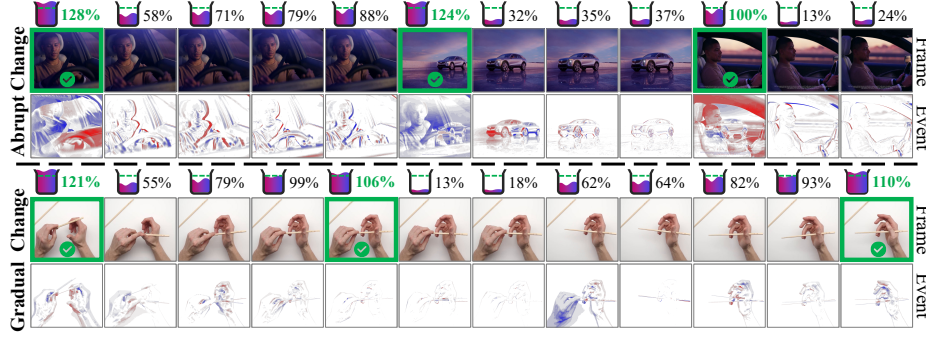
Fig. 4: Visualization of event-accumulation sampling in C2FS. After each sampling step, the accumulated event value is reduced by the threshold (100%). The two examples illustrate that redundant frames are effectively filtered out.
