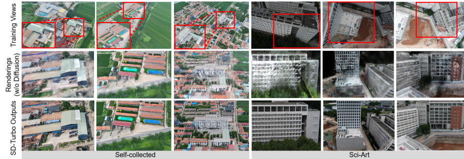
Fig. 9: Visual comparison of unobserved facade generation. The top row shows the top-down aerial images used for training. The middle row illustrates the novel side-view rendering results without diffusion guidance, while the bottom row demonstrates the results directly generated by SD-Turbo.
