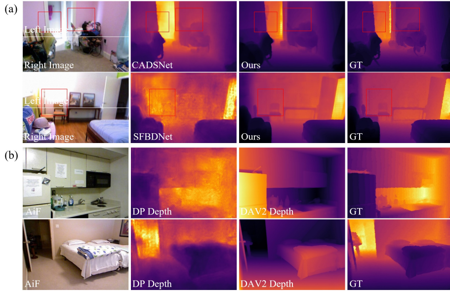
Fig. 1: (a) Qualitative comparison. Our method yields sharper boundaries and more accurate depth in weak-disparity regions (highlighted in red). (b) Complementary failure modes: DPNet preserves metric scale but degrades structurally, while DAV2 recovers structure but lacks metric scale. Best viewed by zooming in.
