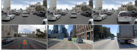
Figure 7: Corner cases. First row: a reversing white van. Second row: a traffic cone ahead of the ego vehicle, a child chasing a ball, and truck swerving into the lane.
