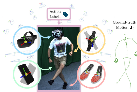
Fig. 2: Wearable capture rig. Two smart insoles (pressure + IMU), two smartwatches and two smartphones (IMUs), and an HMD (6-DoF pose), all synchronized with markerless MoCap.
