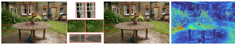
Fig. 2: Visual example of reconstruction residual on training views. (Left) ground truth, (Center) rendering, (Right) residual map. The residual maps capture errors caused by both imperfect geometry ( e.g. , under-reconstructed regions in vegetation) and the limited capacity of view-dependent appearance ( e.g. , reflections on the table).
