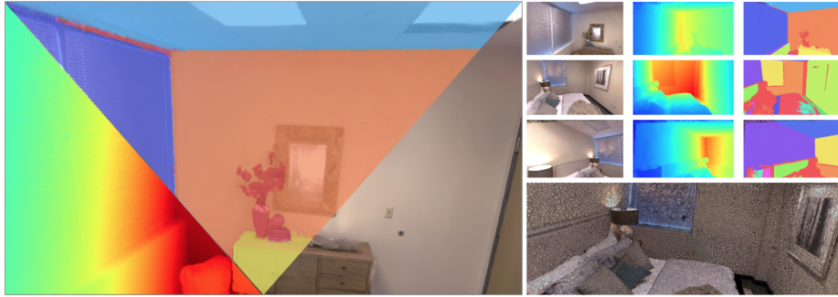
Fig. 1: Example results from the proposed Structure Gaussian Splatting SLAM system. The left part visualizes the reconstructed 3D scene in depth, plane-instance, and appearance formats; the top-right shows novel-view synthesis during tracking; and the bottom-right displays the reconstructed 3D Gaussian primitives of the scene.
