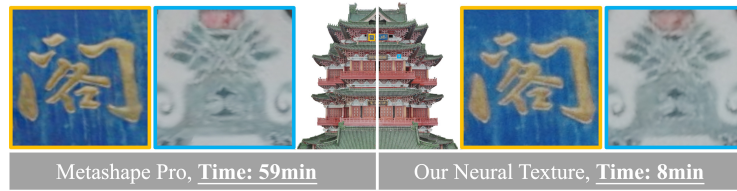
Fig. 10: Run time comparison with Metashape Pro [45] in terms of mesh texturing. Our method demonstrates comparable visual quality while achieving over 7\times acceleration.
