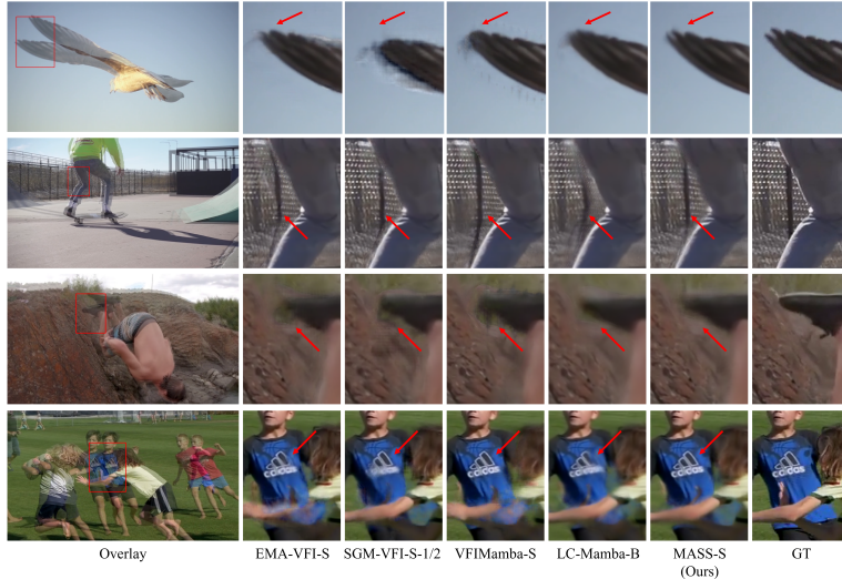
Fig. 4: Visual comparison on SNU-FILM [3]. The red arrows highlight regions with large motions and fine details.
