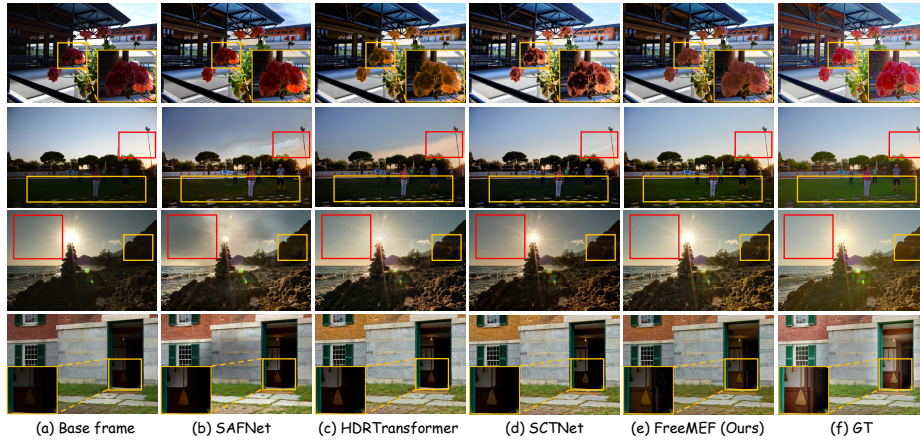
Fig. 6: Visual comparisons between models trained on Kalantari et al. 's dataset [27] and tested on the SICE dataset [5]. Under-exposed and over-exposed regions are marked with yellow and red boxes, respectively. Our method achieves a higher dynamic range and consistently delivers superior visual quality. Zoom in for a better view. Note that Kalantari et al. 's training dataset [27] contains fewer exposure levels than SICE [5], resulting in a lower dynamic range of all model outputs compared to the ground truth.
