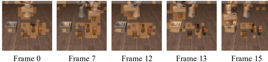
Fig. 3: Visualization of semantic attention consistency and subtask transitions. We visualize key attention tokens (orange) across five frames of a robotic pick-and-place episode. For most steps, attention remains anchored to task-relevant semantic entities rather than spatial positions, demonstrating semantic consistency. An abrupt shift in attention occurs at Frame 13, which coincides with the subtask transition. This temporal evolution highlights both the stability of semantic attention within a subtask and the abrupt shift at the boundary between two distinct subtasks.
