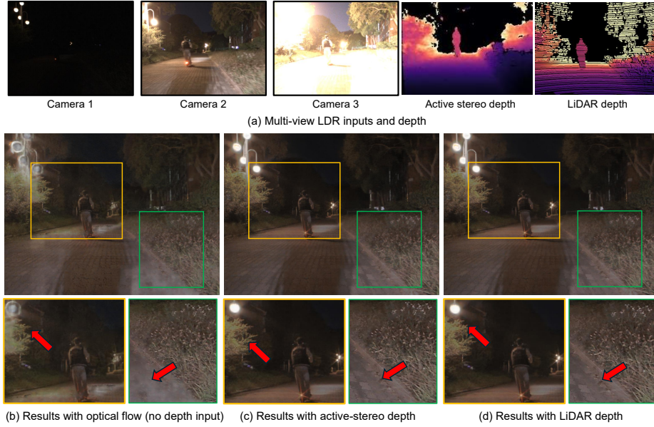
Fig. 5: Importance of depth and evaluation with different depth modalities. DMEB provides robust reconstruction accuracy using either active-stereo or LiDAR depth. However, when depth is not provided and optical flow is used instead for photometric matching, HDR reconstruction fails due to the drastically different exposure gaps between cameras.
