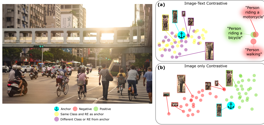
Fig. 2: Existing REC methods [19, 67] rely on image-text contrastive learning approaches that depend on text guidance, which can introduce misalignment and limit fine-grained separation between visually similar instances. (a) Each anchor visual token (in blue) is compared to the positive (green) and negative (red) prompt text embeddings. The image and text embedding spaces are not necessarily aligned which can lead to the visual tokens that correspond to those different prompts to be entangled, as they are not separated directly. (b) Instead, we propose performing image-only contrastive learning, directly optimizing relationships among object embeddings in the visual space. This yields more compact intra-class clusters and clearer inter-class separation, improving discrimination between visually and contextually distinct objects.
