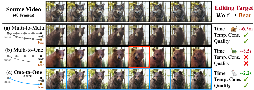
Fig. 1: Three frameworks for text-guided video editing. (a) Multi-to-Multi : The standard approach yields high-quality edits but is impractically slow. (b) Multi-to-One : Naïvely adopting a one-step diffusion model produces degraded, temporally inconsistent outputs. (c) One-to-One (Ours) : Our proposed framework uses a learnable one-step encoder to enable fast, temporally consistent, and high-quality video editing, resolving the speed-quality trade-off.
