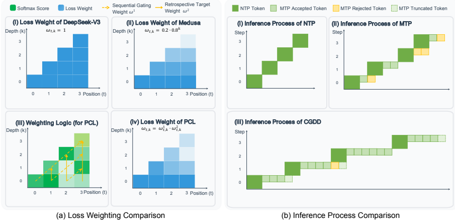
Fig. 1: Comparative illustration of P-MTP training and inference, where (a) shows a comparison of different MTP weighting schemes and (b) shows a comparison of drafting paradigms. In (a), unlike the constant weights in (i) DeepSeek-V3 or static decay in (ii) Medusa, P-MTP introduce Progressive Curriculum Loss which weights look-ahead depths adaptively via (\omega^1, \omega^2) . In (b), compared to (i) NTP and (ii) fixed-depth MTP, (iii) P-MTP adaptively extends the drafting depth using confidence-gating, maximizing accepted tokens while truncating unreliable paths.
